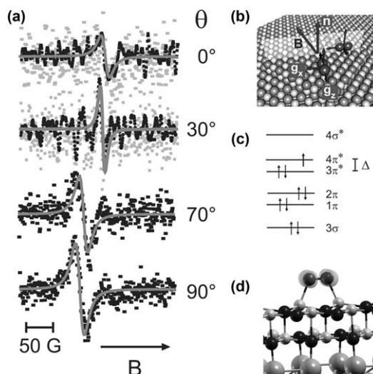
**Fig. 3** (a) Angular dependent EPR spectra of  $\text{O}_2^{\bullet-}$  radicals spontaneously formed on 4 ML thick stoichiometric  $\text{MgO}(001)$  film on  $\text{Mo}(001)$ . (b) Schematics of the experimental geometry. (c) Schematic MO diagram of an  $\text{O}_2^{\bullet-}$  radical. (d) Binding geometry as calculated theoretically.
