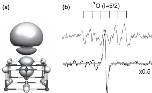
**Fig. 2** (a) Calculated spin density of Au atoms adsorbed on oxygen ions of a MgO(001) surface. (b) EPR signal of the most intense line from Fig. 1a (bottom trace) and spectrum found after growth of a  $^{17}\text{O}$  enriched MgO(001) film (top trace).
